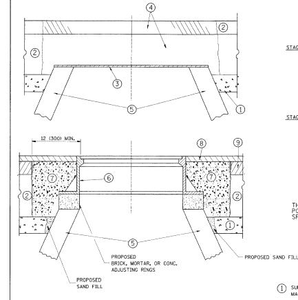
EXISTING BROKEN FRAMES AND LIDS SHALL BE REMOVED AND DISPOSED OF BY THE CONTRACTOR AND SHALL BE REPLACED AS DIRECTED BY THE ENCINEER, REPLACEMENT FRAMES AND LIDS WILL BE PAID FOR IN ACCORDANCE WITH ARTICLE 103,04 OF THE STANDARD SPECIFICATIONS UNLESS A SEPARATE PAY ITEM HAS BEEN PROVIDED.
