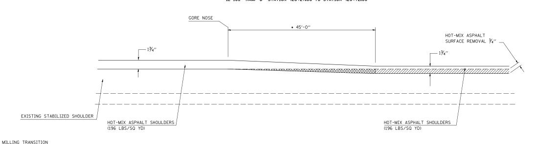
AREA OF MILLING TRANSITION SHALL BE INCLUDED IN CONTRACT UNIT PRICE FOR THE HOT-MIX ASPHALT SURFACE REMOVAL - 3/4". NO ADDITIONAL
