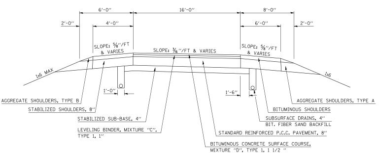
NOTE: MAXIMUM SUPERELEVATION ≤ 0.08 FT/FT ALGEBRAIC DIFFERENCE BETWEEN PAVEMENT AND SHOULDER ≤ 0.08 FT/FT
