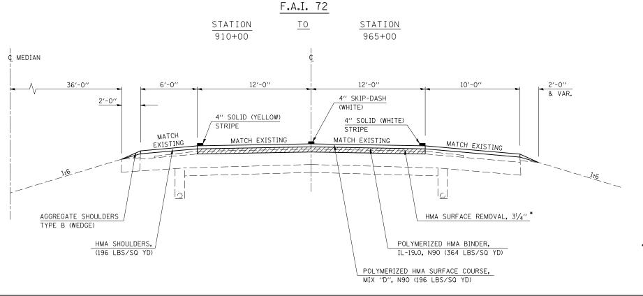
\*THE SPECIFIED DEPTH IS INTENDED TO REMOVE THE FULL THICKNESS OF EXISTING HMA OVERLAY AND TEXTURE THE EXISTING CONCRETE PAVEMENT SURFACE.
