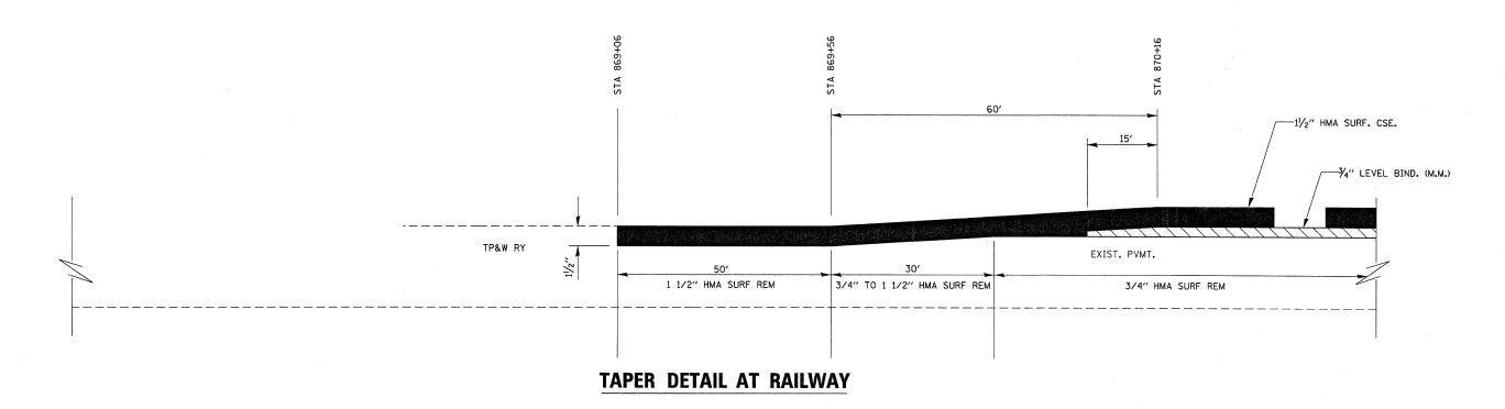
NOTE: HMA SURFACE REMOVAL TRANSITION AND HMA SURFACE REMOVAL, 1 1/12" WILL BE PAID FOR AS HMA SURFACE REMOVAL 3/4"
