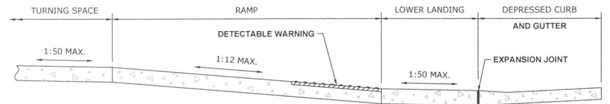
THE RUNNING SLOPE OF THE CURB RAMP SHALL NOT REQUIRE THE CURB LENGTH TO EXCEED 15'.
