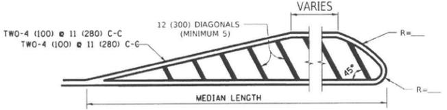
FOR MEDIAN LENGTHS WHERE DIAGONAL SPACING CANNOT BE ATTAINED, USE 5 (FIVE) EQUALLY SPACED DIAGONAL LINES.
