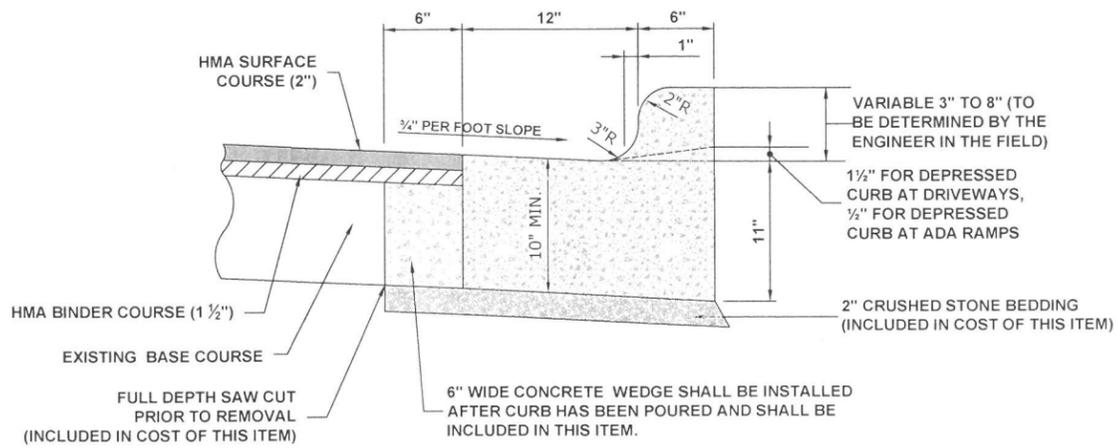
**COMBINATION CONCRETE CURB & GUTTER TYPE B-6.12 (MODIFIED)**
