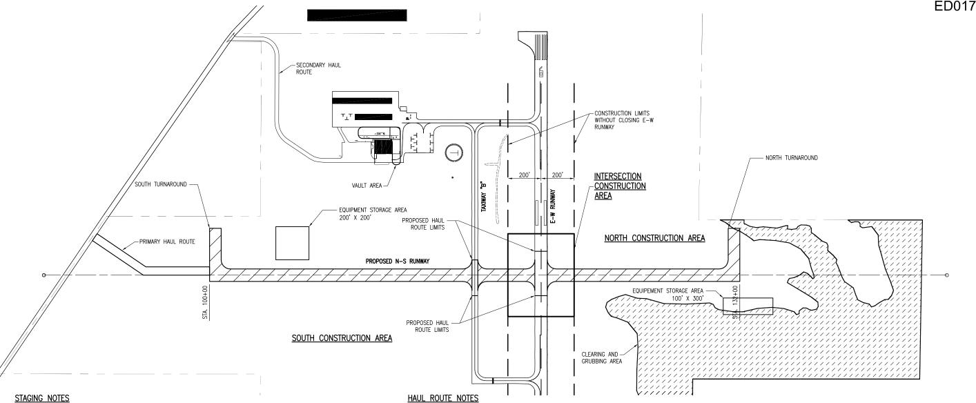
THE INTENT OF THIS STAGING OR SEQUENCING PLAN IS TO ACT AS A PROCEDURAL GUIDE TO ACCOMPLISH THE WORK IN A TIMELY MATTER WHILE KEEPING THE E-W RUNWAY OPEN AND HENCE THE AIRPORT OPEN AS MUCH AS POSSIBLE. EVERY EFFORT SHOULD BE MADE TO KEEP THE E-W RUNWAY OPEN FOR OPERATIONS.
