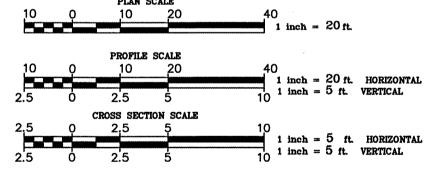
FULL SIZED PLANS HAVE BEEN PREPARED USING STANDARD ENGINEERING SCALES. REDUCED—SIZED PLANS WILL NOT CONFORM TO STANARD SCALES. IN MARKING MEASUREMENTS ON REDUCED SIZE PLANS, THE ABOVE SCALES MAY BE USED.
