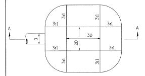
D= INSIDE DIAMETER OF PIPE CULVERT OR CLEAR WIDTH OF BOX CULVERT
