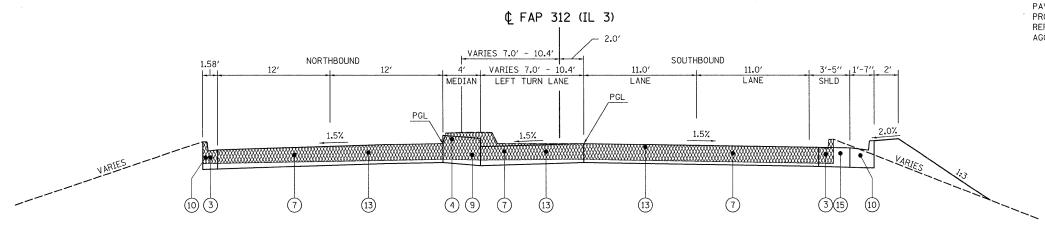
NOTE: WHERE PROPOSED REMOVAL OF EXISTING PAVEMENT OR CURB/MEDIAN IS REQUIRED BELOW THE PROPOSED PORTLAND CEMENT CONCRETE PAVEMENT, REPLACE REMOVED MATERIAL WITH PROPOSED AGGREGATE BASE COURSE, TYPE A
