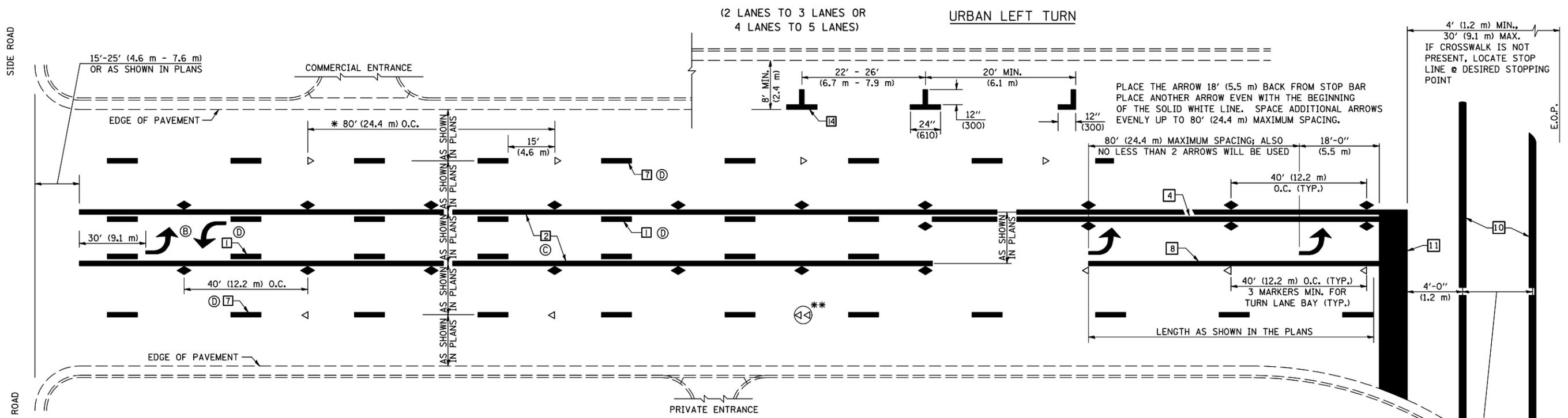
\* REDUCE TO 40 FEET (12.2 METERS) ON CENTER ON CURVES WHERE ADVISORY SPEEDS ARE 10 MPH (15 km/h) LOWER THAN POSTED SPEEDS.
