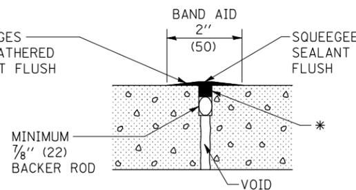
\* HOT ASPHALT CRACK SEALANT APPROX. 3/4 \"
