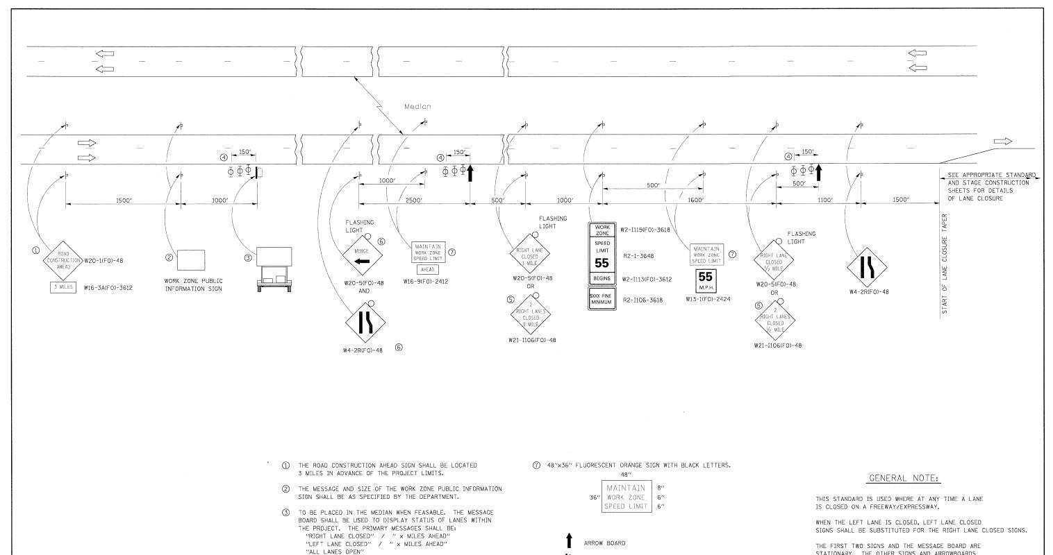
THE FIRST TWO SIGNS AND THE MESSAGE BOARD ARE STATIONARY. THE OTHER SIGNS AND ARROWBOARDS SHALL BE MOVED AS NECESSARY TO MAINTAIN THE REQUIRED DISTANCE FROM THE START OF THE LANE CLOSURE TAPER(S).
