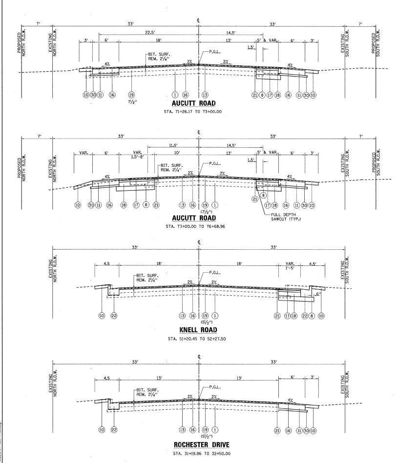
STRUCTURAL DESIGN TRAFFIC: Year 2025 PV = 8460SU = 225 MU = 315Class <u>II</u> ROAD/STREET CLASSIFICATION: PERCENT OF STRUCTURAL DESIGN TRAFFIC IN DESIGN LANE: P = 50 % S = 50 % M = 50 % TRAFFIC FACTOR: Actual TF = 1.48 AC Type = PG 64-22 (AC-20)Minimum TF = 0.5PG GRADE: Binder = PG64-22 Surface = PG64-22 SUBGRADE SUPPORT RATING:
