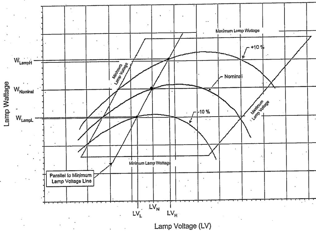
$$\text{Ballast Regulation} = \frac{W_{LampH} - W_{LampL}}{W_{LampN}} \times 100$$
