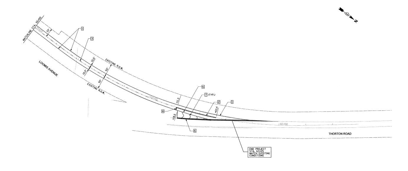
HOT-MIX ASPHALT SURFACE REMOVAL BUTT JOINT, TEMPORARY RAMPS
