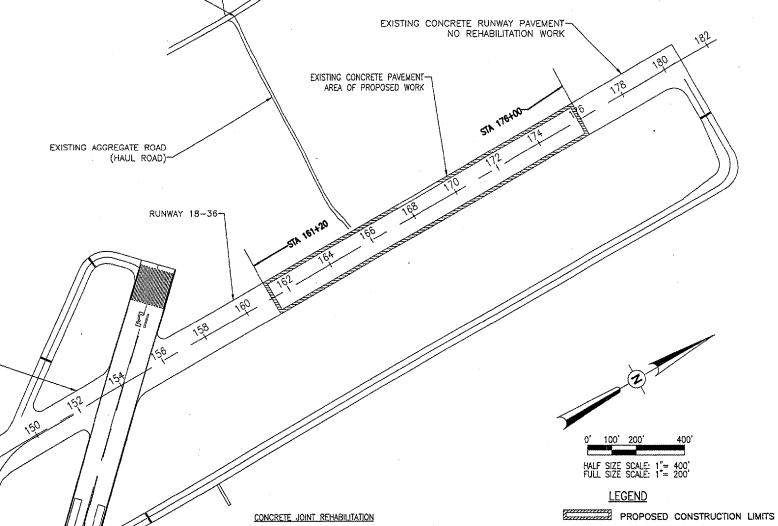
CONCRETE JOINT REHABILITATION SHALL CONSIST OF REMOVAL OF
