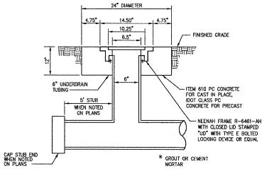
UNDERDRAIN INSPECTION HOLE
