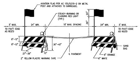
BARRICADES ARE TO BE OF IDOT TYPE I. A STEADY-BURNING OR FLASHING RED LIGHT FACING PASSING TRAFFIC IS TO BE MOUNTED ABOVE THE TOP OF EACH BARRICADE FRAME. THE BARRICADE IS TO BE STABILIZED FROM WIND BY SANDBAGS PLACED ON THE FRAME OR OTHER METHODS APPROVED BY THE RESIDENT ENGINEER. NO PART OF THE REFLECTORIZED PORTION OF THE BARRICADE IS TO BE OBSTRUCTED IN ANY MANNER. COST OF FURNISHING, INSTALLING, RELOCATING AND MAINTAINING BARRICADES IS TO BE INCIDENTAL TO THE CONTRACT.
