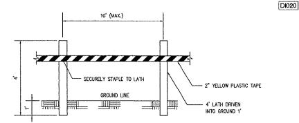
MATERIALS ARE TO BE APPROVED BY ENGINEER PRIOR TO INSTALLATION. COST OF MATERIALS, INSTALLATION, RELOCATION AND MAINTENANCE OF LATHING AND WARNING TAPE IS TO BE INCIDENTAL TO THE CONTRACT.
