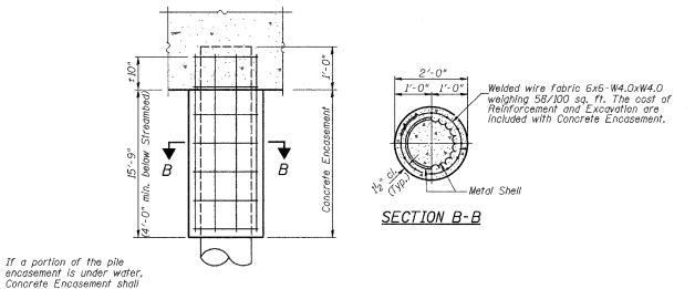
DETAIL OF METAL SHELL PILE ENCASEMENT AT PIERS
