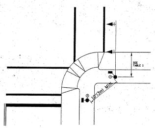
RECOMMENDED PUSHBUTTON LOCATIONS FOR ACCESSIBLE PEDESTRIAN SIGNALS SHALL BE IN ACCORDANCE WITH THE CURRENT MUTCD (SEE NOTE 1). TO MEET MUTCD REQUIREMENTS, PEDESTRIAN SIGNAL PUSHBUTTONS MAY HAVE TO BE 7 MOUNTED ON A SEPARATE POST.
