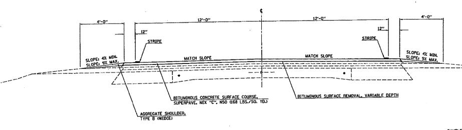
JUDGEMENT SHOULD BE EXCERCISED DURING PROFILE MILLING. THE INTENT OF THE MILLING OPERATION IS TO ESTABLISH A NOMINAL %"/FT. SLOPE, REMOVE HIGH BUMPS AND REMOVE MOST OF THE RUTTING. (SEE SPECIAL PROVISIONS)
