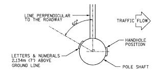
POSITION OF HANDHOLE AND POLE NUMBER FOR IN-FIELD POLES
