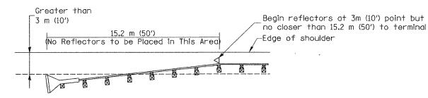
NOTE: Omit terminal marker when terminal over (10') from edge of paved shoulder or break point of unpaved shoulder.
