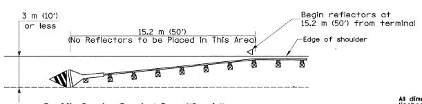
Traffic Barrier Terminal Type 1(Specia) [Terminal 3 m (10') or less from edge of shoulder] All dimensions are in millimeters (inches) unless otherwise noted. ILLINOIS DEPARTMENT OF TRANSPORTATION
