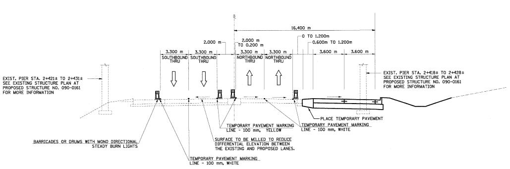
NORTH MAIN ST MOT TYPICAL SECTION NO. 6A STA. 2+412.933 TO STA. 2+579.299
