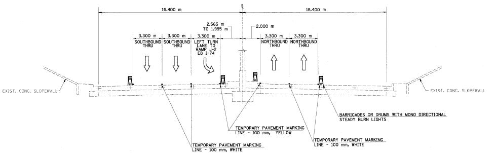
NORTH MAIN ST MOT TYPICAL SECTION NO. 5A
