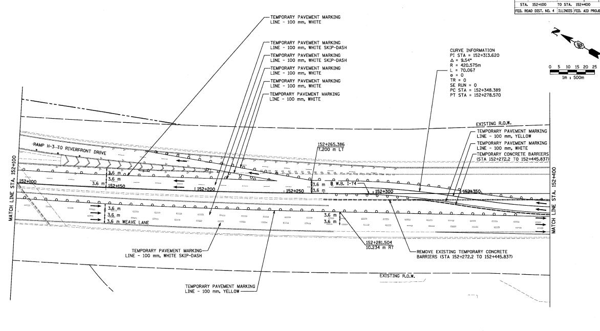
LEGEND TEMPORARY PAVEMENT MARKING TRAFFIC FLOW DIRECTION o DRUM WITH STEADY BURNING MONO-DIRECTIONAL LIGHT ---- TEMPORARY CONCRETE BARRIER
