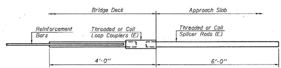
**FOR INTEGRAL OR SEMI-INTEGRAL ABUTMENTS**
