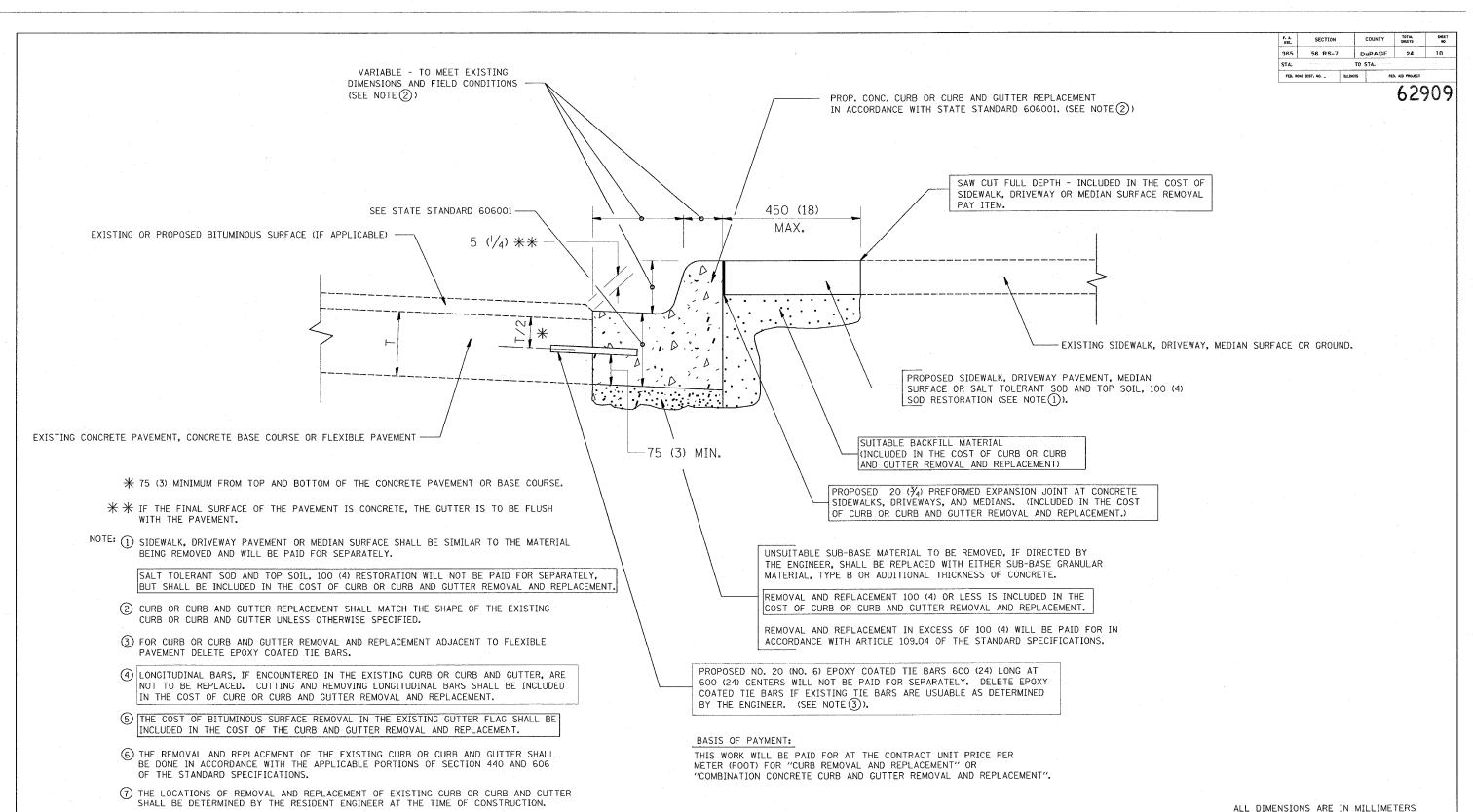
CURB OR CURB AND GUTTER REMOVAL AND REPLACEMENT
