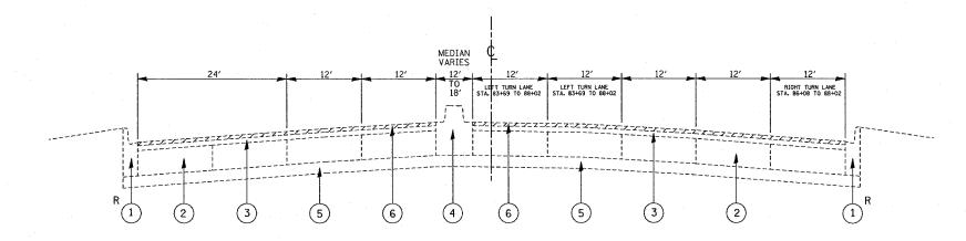
EXISTING TYPICAL CROSS SECTION STA. 83+30 TO 88+29
