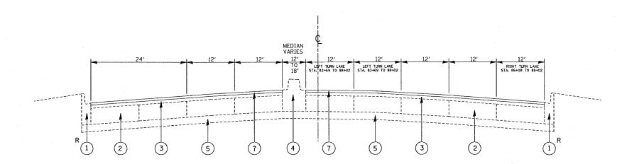
PROPOSED TYPICAL CROSS SECTION STA. 83+30 TO 88+29
