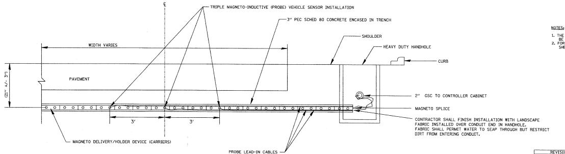
DAN RYAN TYPICAL SINGLE LANE EXIT/ENTRANCE MULTI MAGNETO-INDUCTIVE VEHICLE SENSOR (PROBE) INSTALLATION
