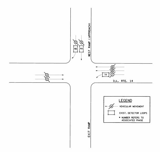
REFERRING TO STANDARD 857001, THE VEHICULAR AND PEDESTRIAN PHASES USED ARE DESIGNATED AS SHOWN.
