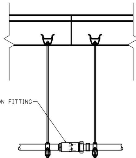
**CONCRETE ATTACHED EXPANSION/DEFLECTION FITTING DETAIL**
