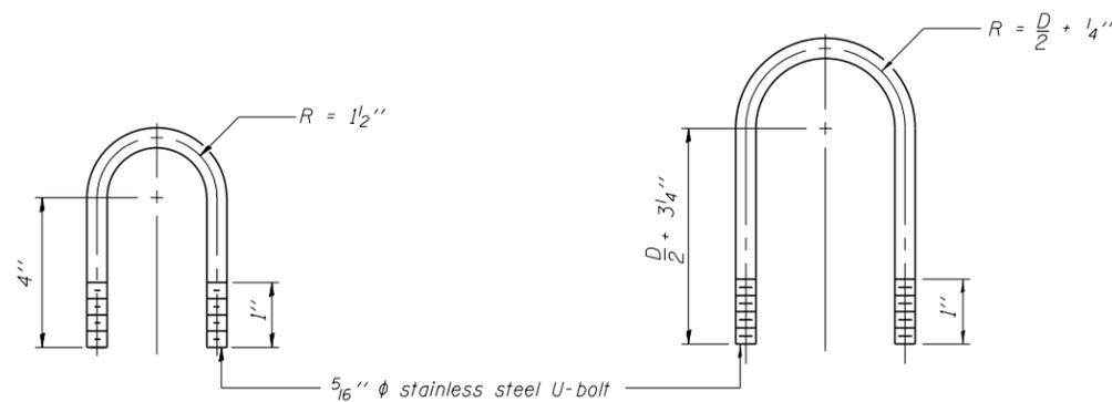
**DAMPING DEVICE MOUNTING TUBE U-BOLT DETAIL**
