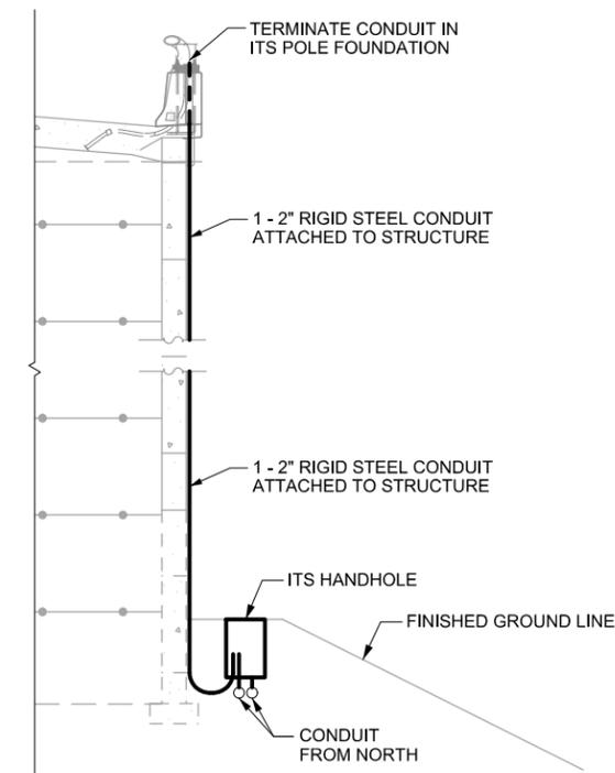
CONDUIT ROUTING UP RETAINING WALL 16
