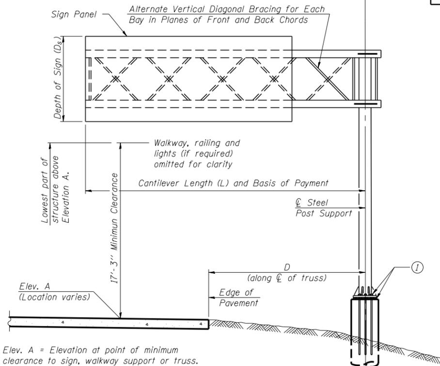
Elev. A = Elevation at point of minimum clearance to sign, walkway support or truss.
