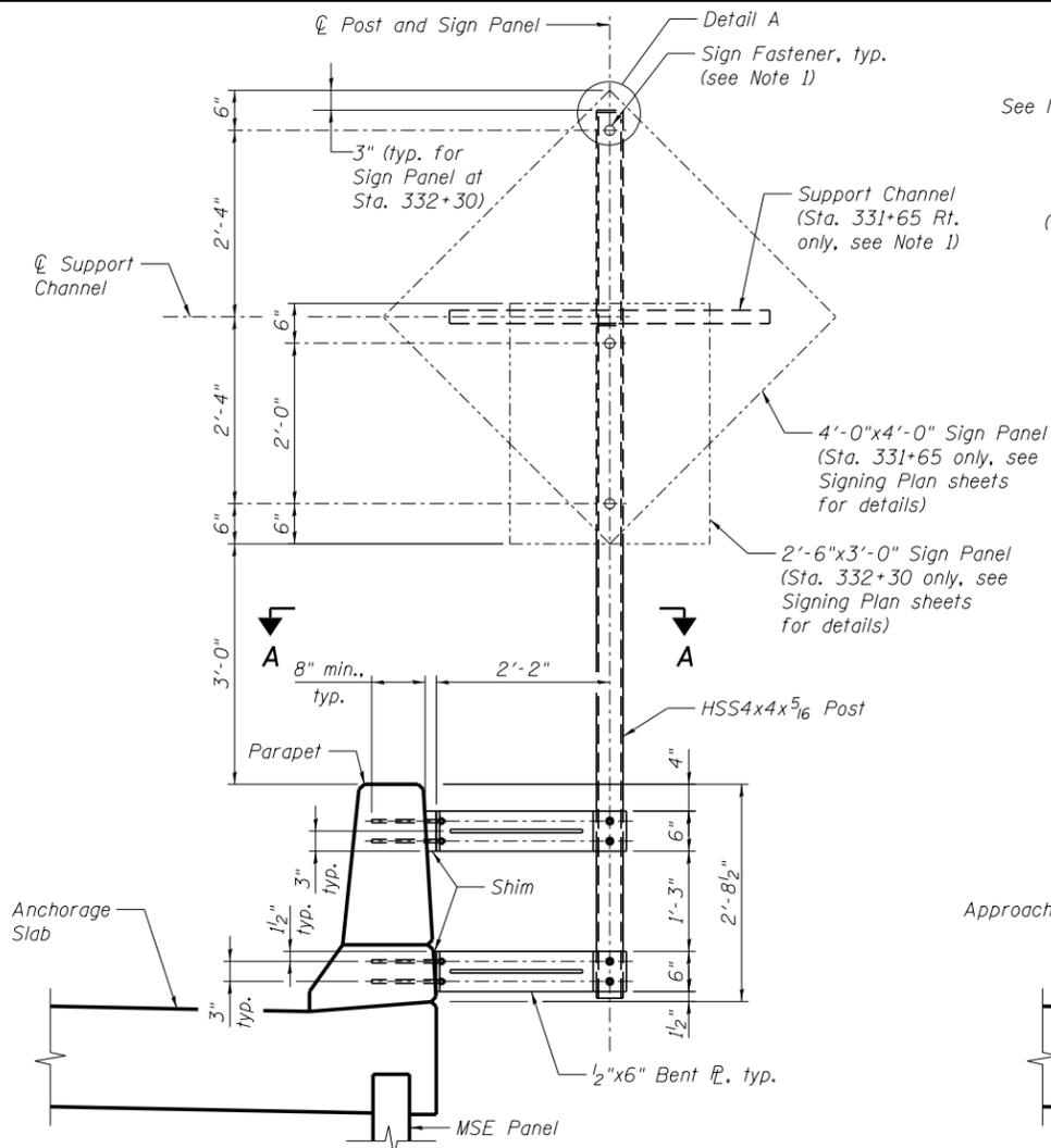
**MSE PARAPET MOUNTED SIGN SUPPORT ASSEMBLY**
