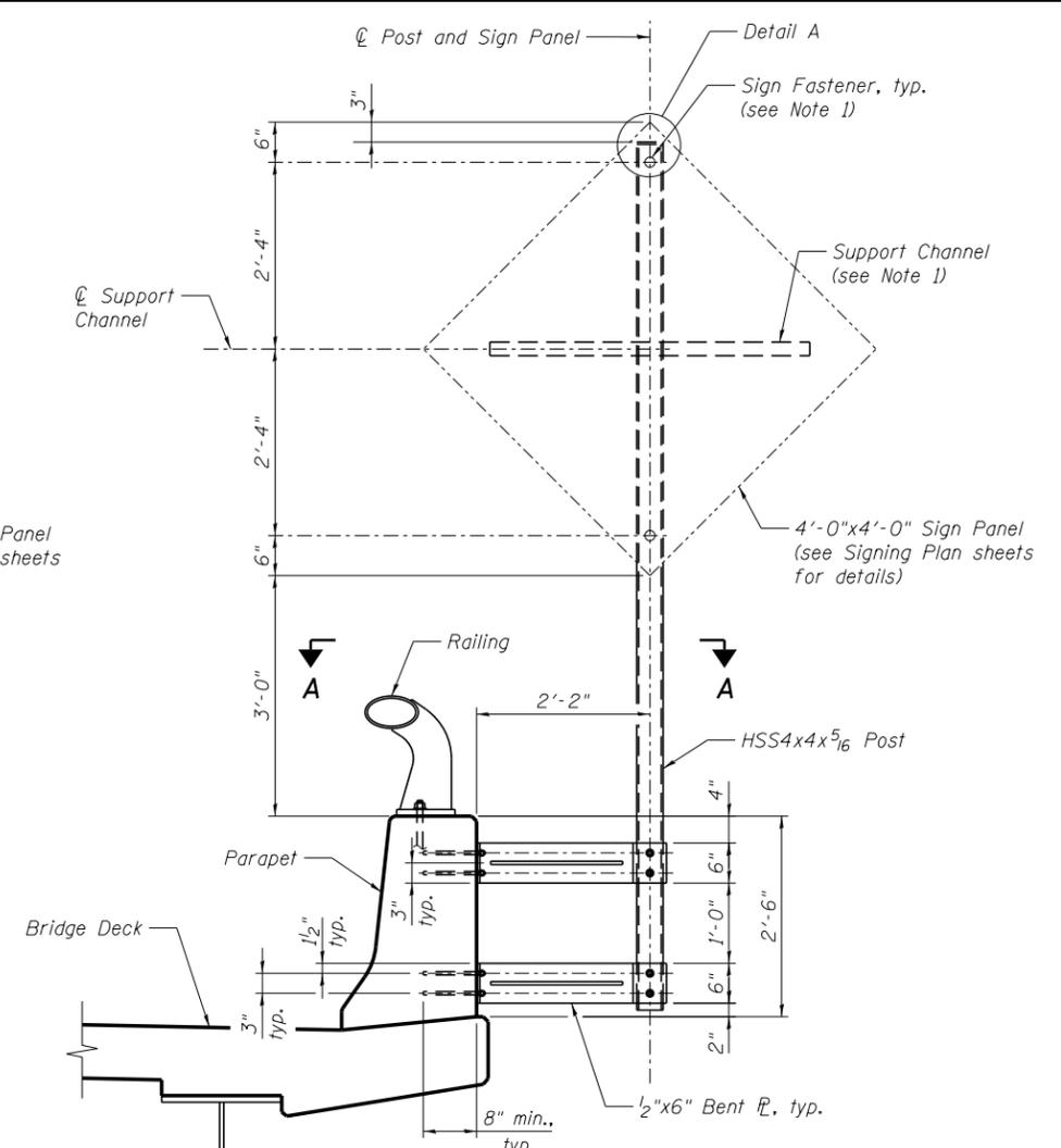
**BRIDGE PARAPET MOUNTED SIGN SUPPORT ASSEMBLY**
