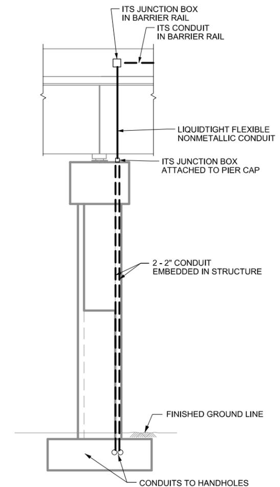
**CONDUIT ROUTING AT PIER 10**
