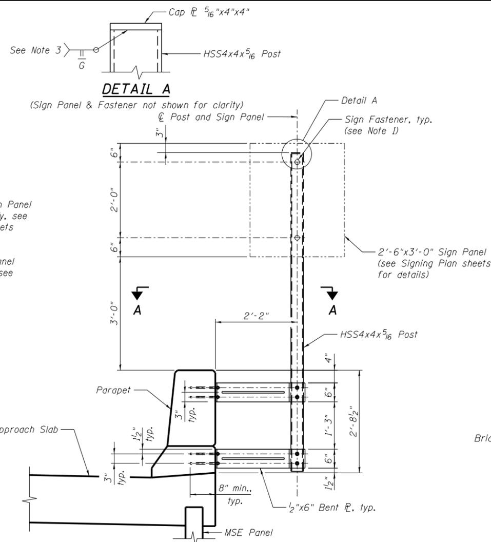
**APPROACH PARAPET MOUNTED SIGN SUPPORT ASSEMBLY**
