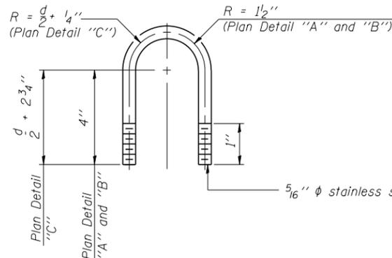
**DAMPING DEVICE MOUNTING TUBE U-BOLT DETAIL**
