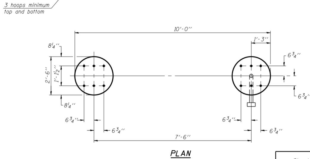
For anchor rod size and placement, see Support Frame Detail Sheet.
