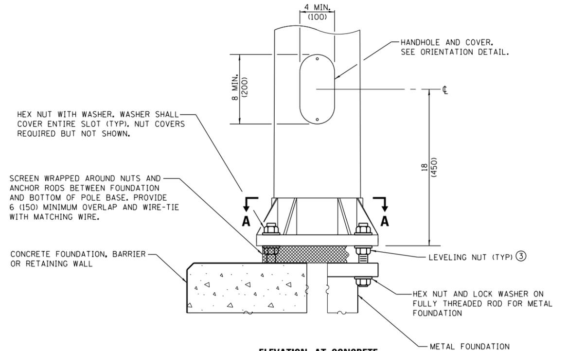
**ELEVATION AT CONCRETE FOUNDATION, METAL FOUNDATION OR RETAINING WALL**
