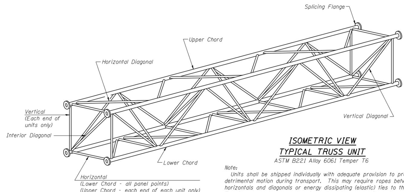
Note: Units shall be shipped individually with adequate provision to prevent detrimental motion during transport. This may require ropes between horizontals and diagonals or energy dissipating (elastic) ties to the vehicle. The Contractor is responsible for maintaining the configuration and protection of the units.
