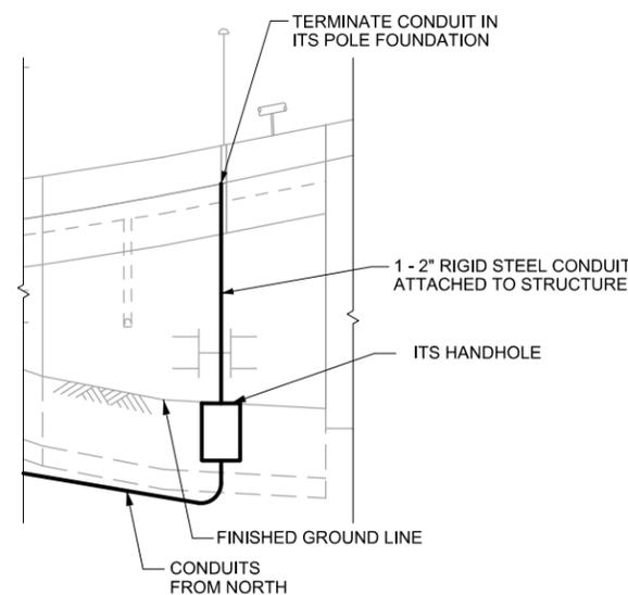
CONDUIT ROUTING UP RETAINING WALL 16
