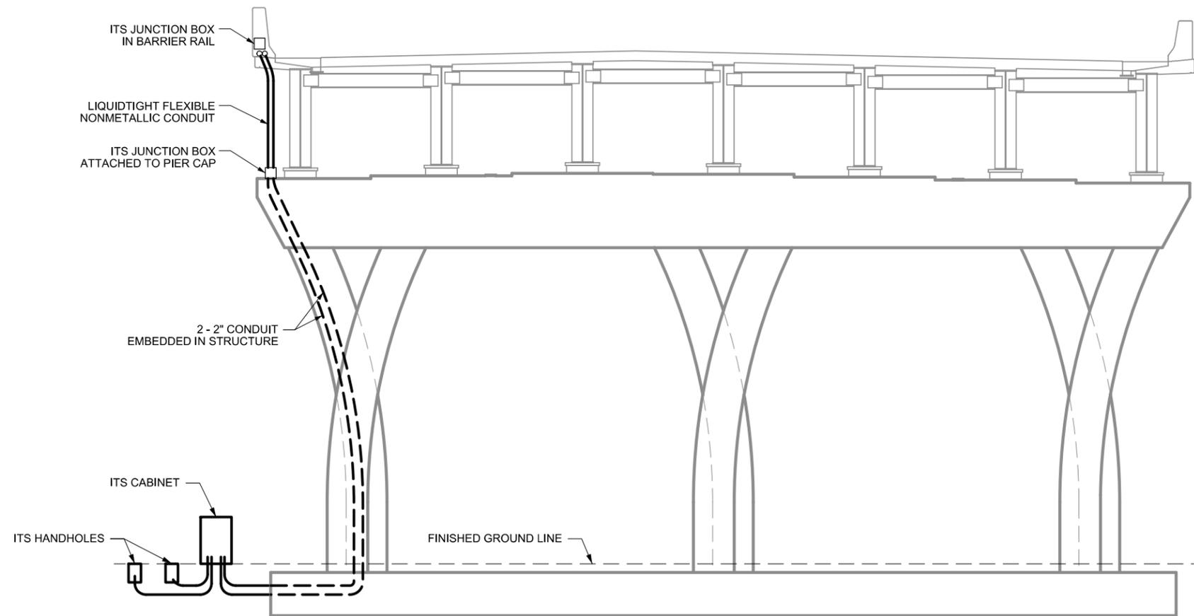
**CONDUIT ROUTING AT PIER 10**
