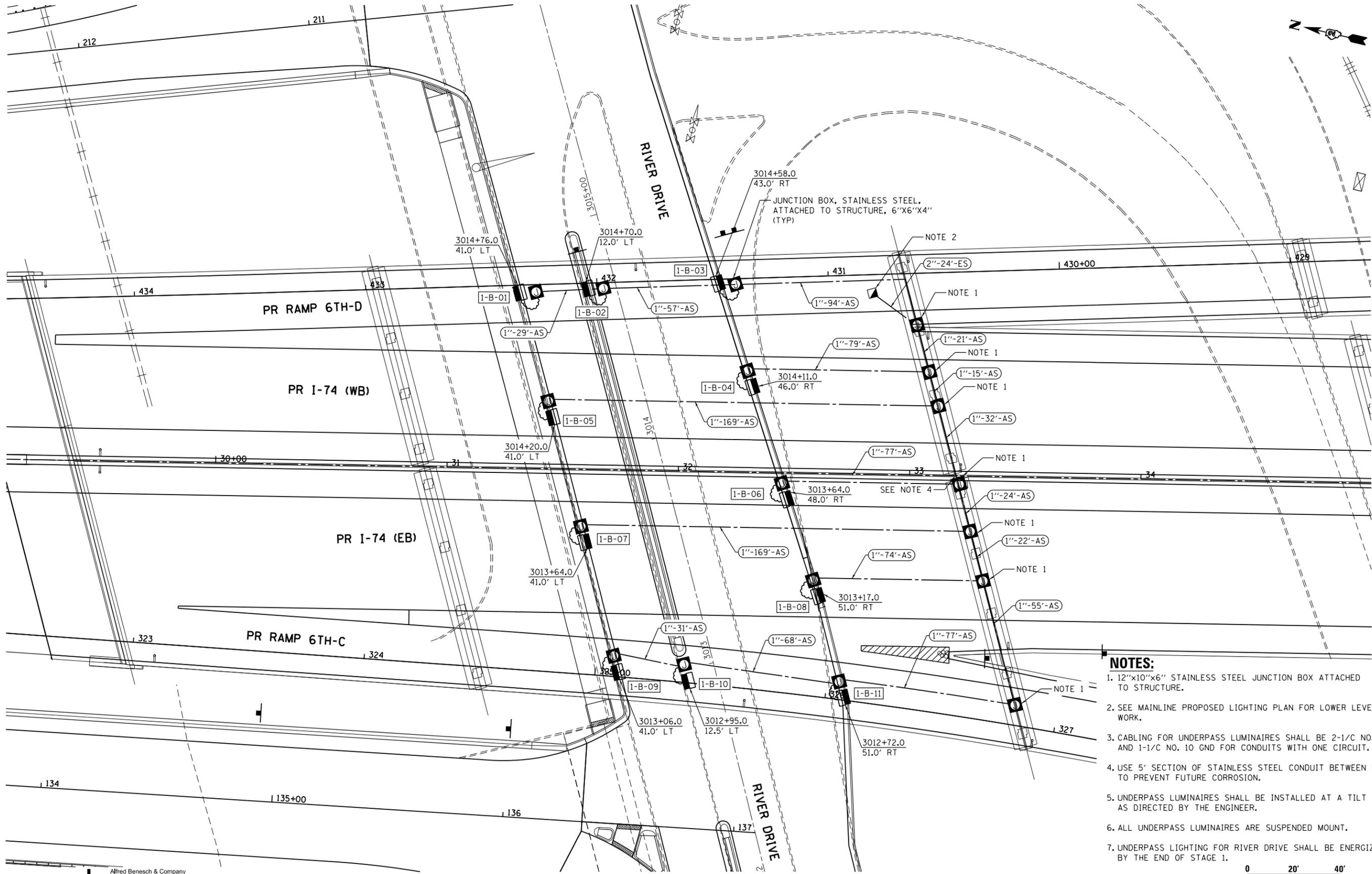
JUNCTION BOX, STAINLESS STEEL, ATTACHED TO STRUCTURE, 6"x6"x4" (TYP)
