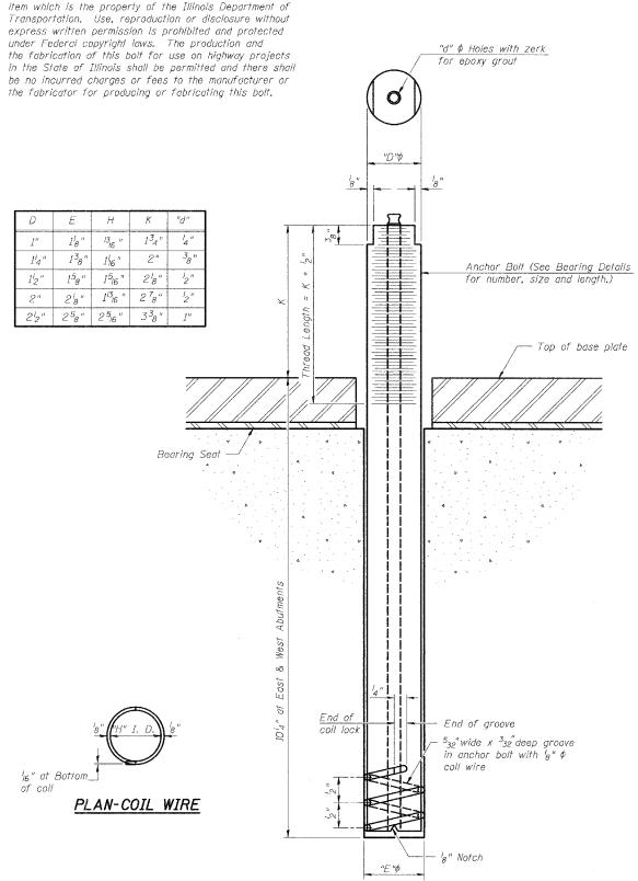
ILLINOIS COIL-LOCK ANCHOR BOLT
