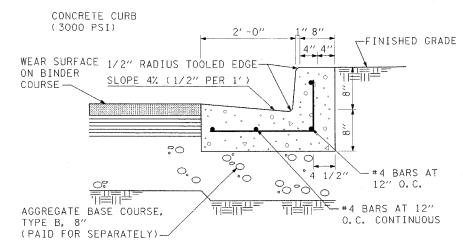
NOTE: PROVIDE CONTROL JOINTS AT 20'-0" OC PROVIDE EXPANSION JOINTS AT 60'-0" OC
