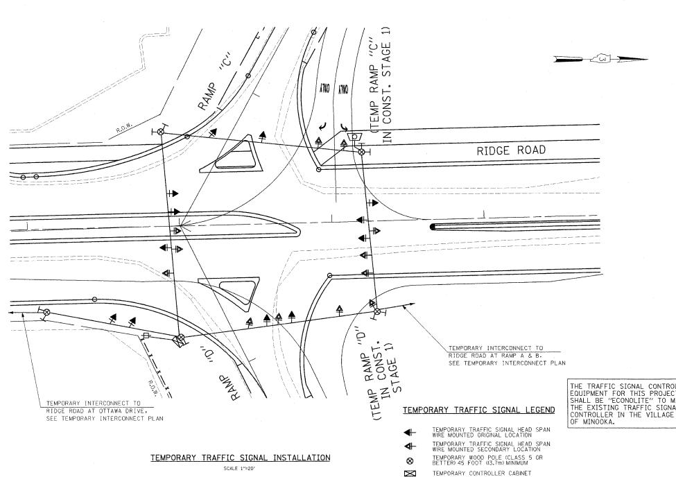
NOTE 1: THE ORIGINAL SIGNAL HEAD PLACEMENT LOCATIONS SHOWN IN THE TEMPORARY TRAFFIC SIGNAL PLAN ARE FOR PRE-STAGE CONSTRUCTION ONLY.
