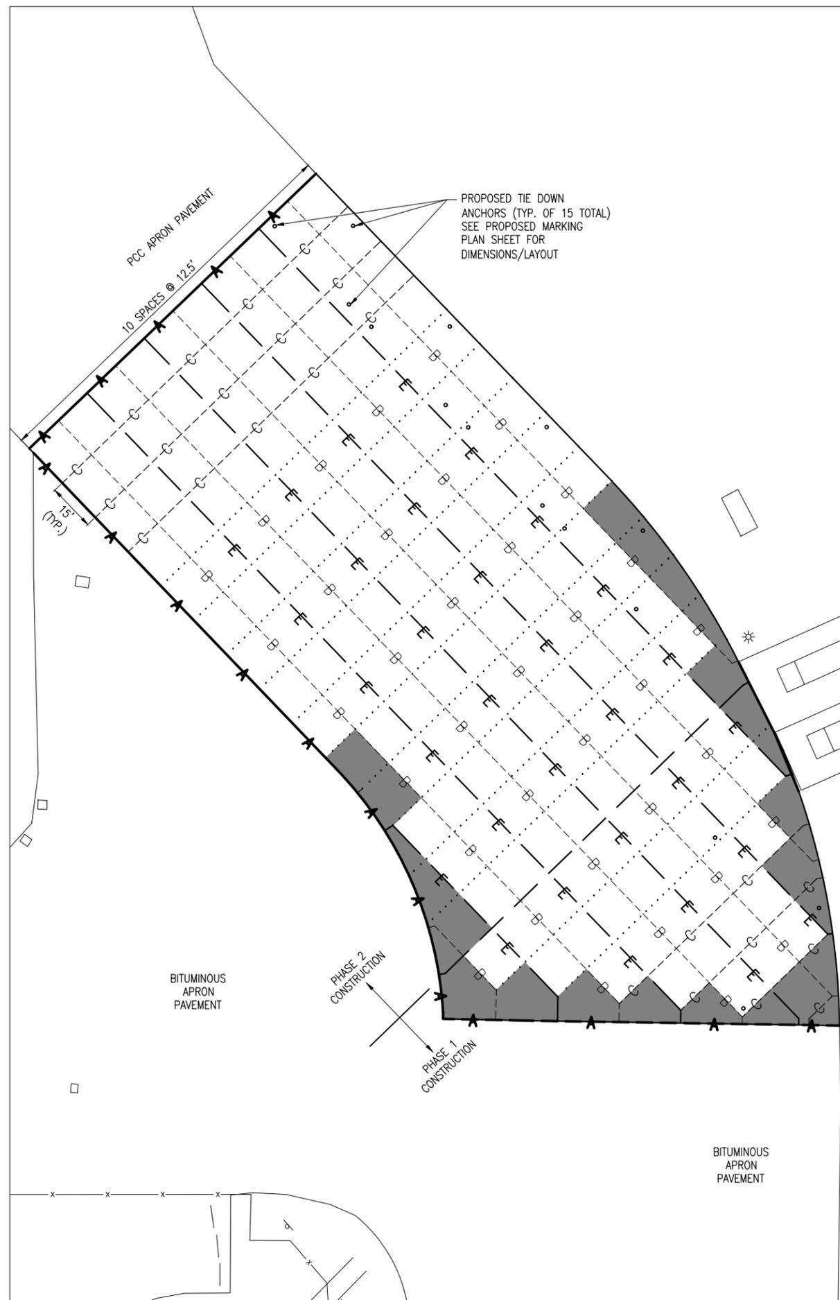
PROPOSED TIE DOWN ANCHORS (TYP. OF 15 TOTAL) SEE PROPOSED MARKING PLAN SHEET FOR DIMENSIONS/LAYOUT
