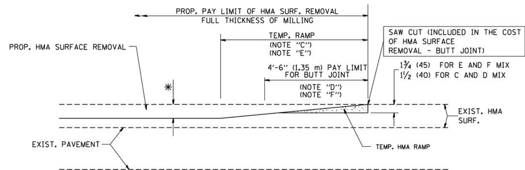
HMA CONSTRUCTED TEMPORARY RAMP
