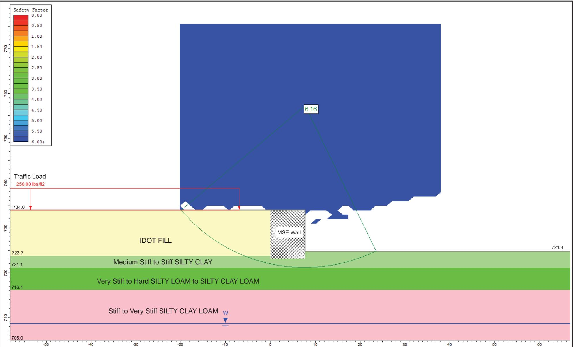
Undrained Analysis for West MSE Wall at Station 134+68.75, Reference Boring BSB2-01
