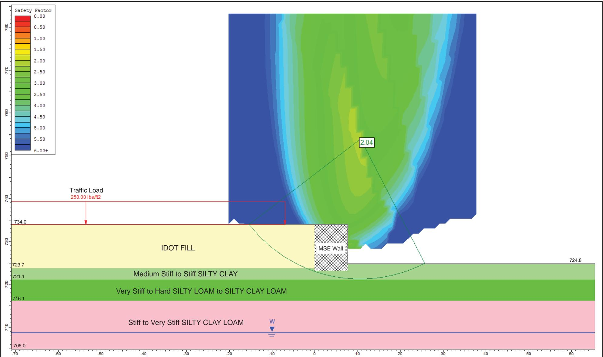
Drained Analysis for West MSE Wall at Station 134+68.75, Reference Boring BSB2-01
