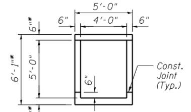
**SECTION THRU BARREL**
