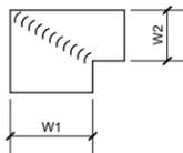
IF W2 DOES NOT EQUAL W1 SPECIAL PROVISIONS MUST BE MADE IN VANE SHAPE OR ANGLE OF ENTRY AND EXIT. APPLIES TO ALL TYPES OF VANES. CONSTRUCT VANE EDGES TO PROJECT TANGENTS PARALLEL TO DUCT SIDES
