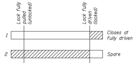
**SPAN AND TAIL LOCK DRIVEN LIMIT SWITCH**
