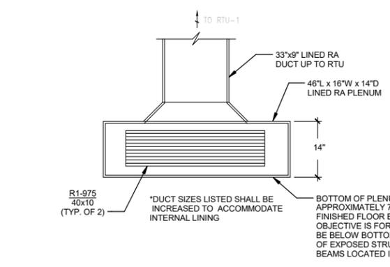
**3 RTU-1 RETURN DUCT EAST ELEVATION**
