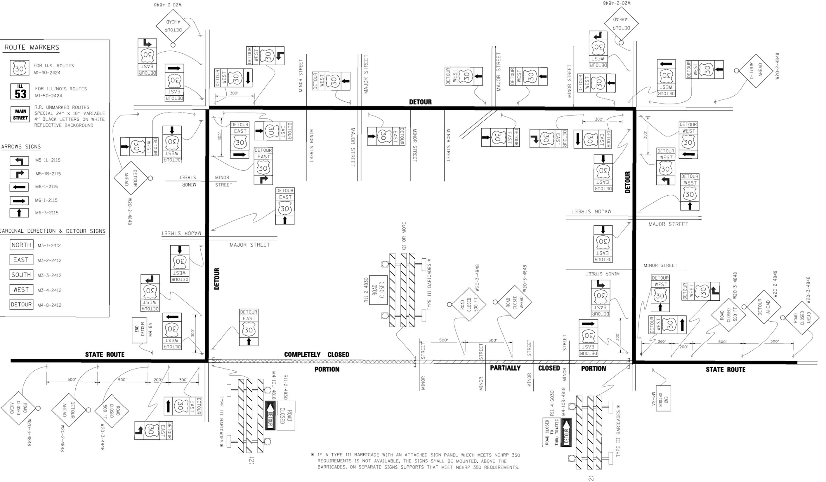
\* IF A TYPE III BARRICADE WITH AN ATTACHED SIGN PANEL WHICH MEETS NCHRP 350 REQUIREMENTS IS NOT AVAILABLE, THE SIGNS SHALL BE MOUNTED, ABOVE THE BARRICADES, ON SEPARATE SIGNS SUPPORTS THAT MEET NCHRP 350 REQUIREMENTS.
