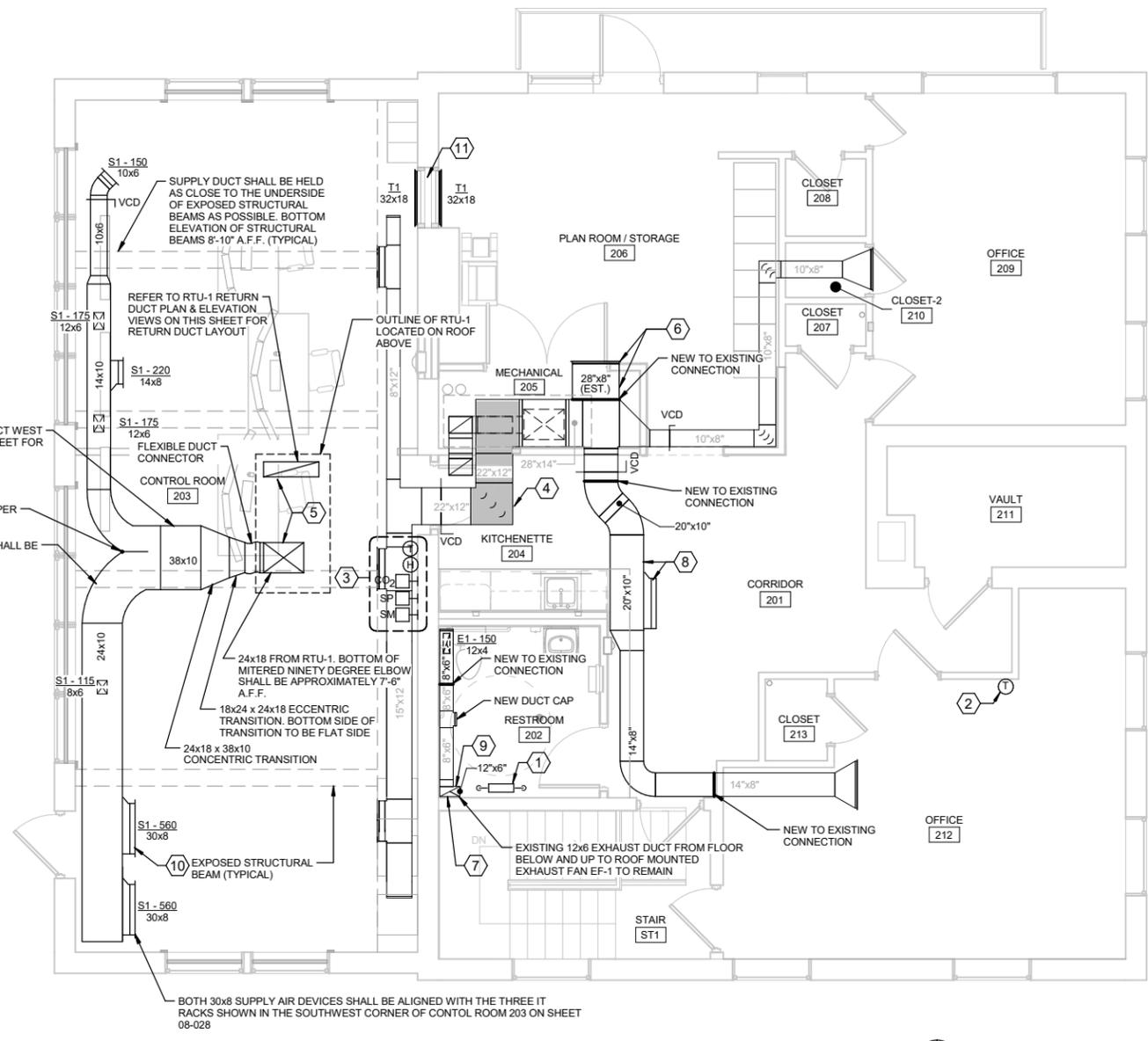
**1 SECOND FLOOR MECHANICAL PLAN - NEW WORK**
