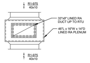
**4 RTU-1 RETURN DUCT PLAN VIEW**
