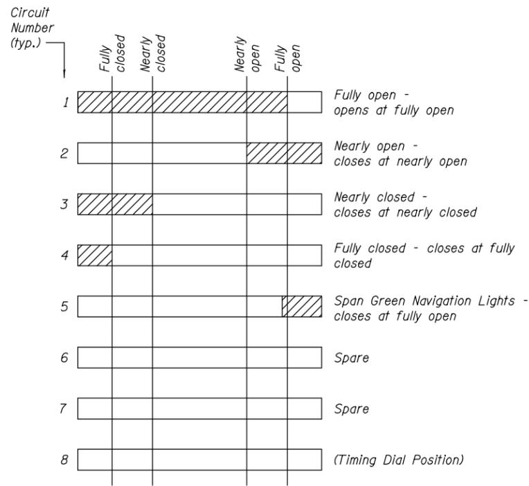
**SPAN CONTROL ROTARY CAM LIMIT SWITCH**
