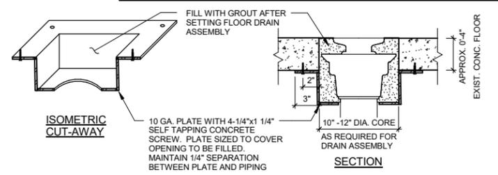
**6 CONCRETE FLOOR PATCHING AT FLOOR DRAIN ASSEMBLY**
