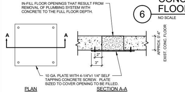
**5 CONCRETE FLOOR PATCHING DETAIL**
