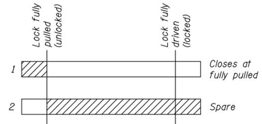
**SPAN AND TAIL LOCK PULLED LIMIT SWITCH**
