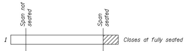
**SPAN FULLY SEATED LIMIT SWITCH**
