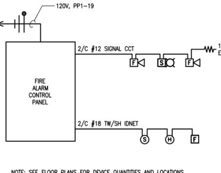
4 TYPICAL FIRE ALARM RISER DIAGRAM
