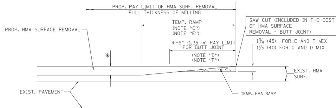
HMA CONSTRUCTED TEMPORARY RAMP
