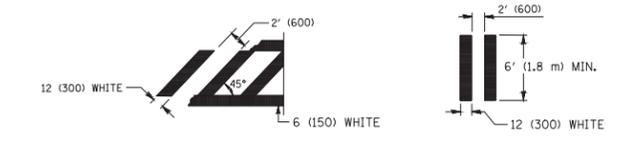
**DETAIL "A" TYPICAL CROSSWALK MARKING**
