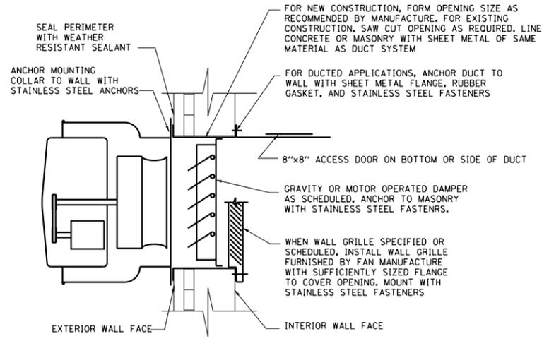
**WALL MOUNTED EXHAUST FAN DETAIL**
