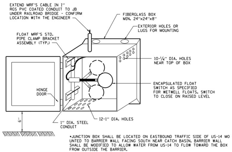
**PAVEMENT FLOODED FLOAT ALARM BOX**
