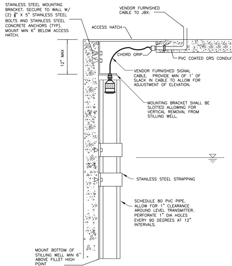
**ULTRASONIC LEVEL SENSOR SIDEWALL STILLING WELL N295**
