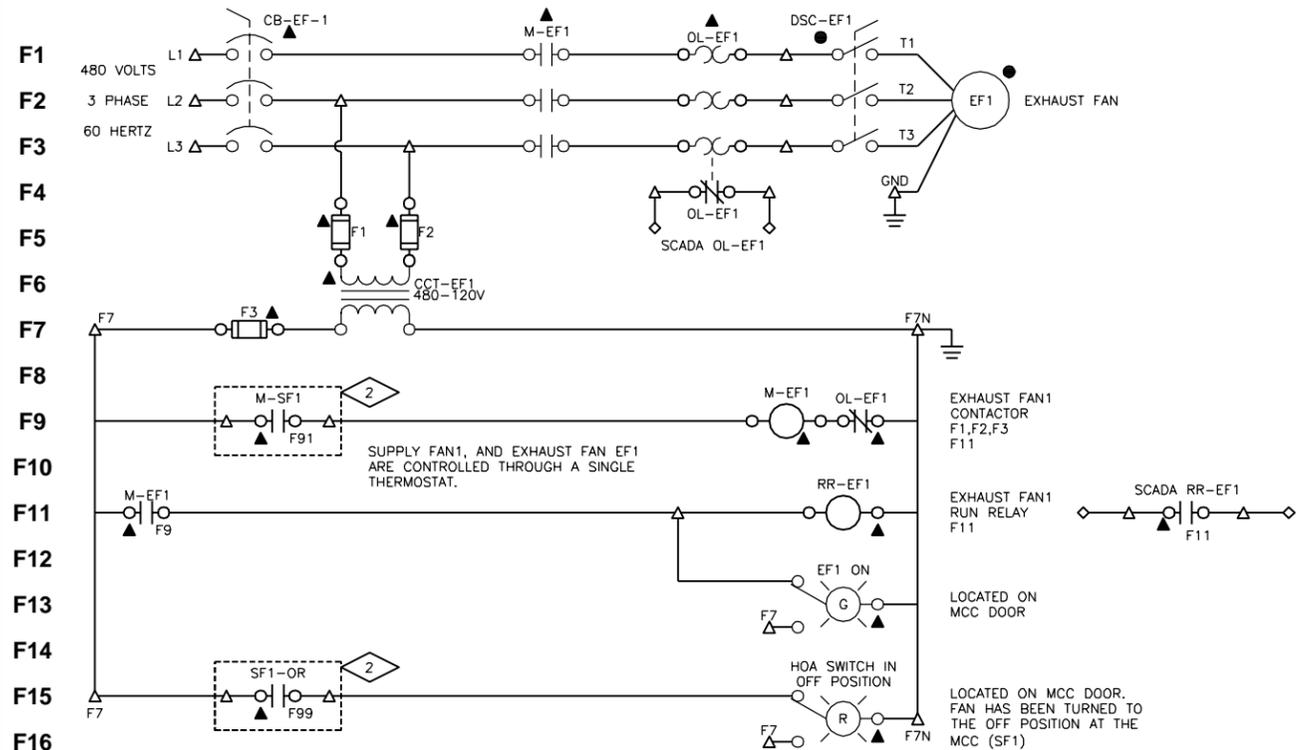
**PUMP STATION EXHAUST FAN - EF1**
