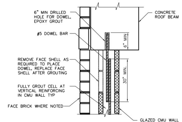
**MASONRY WALL ANCHOR AT ROOF BEAM DETAIL-S36**
