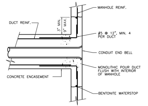
**DUCT PRECAST MANHOLE INTERFACE DETAIL E603**
