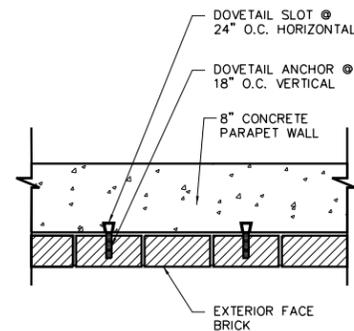
**PARAPET WALL ANCHOR DETAIL-S35**
