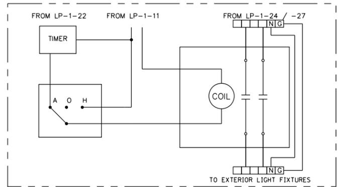
NOTE: NEMA 1 CONTACTOR WITH H-O-A SWITCH ON OUTER ENCLOSURE. TIME SHALL UTILIZE ASTRONOMICAL TIME SWITCH.
