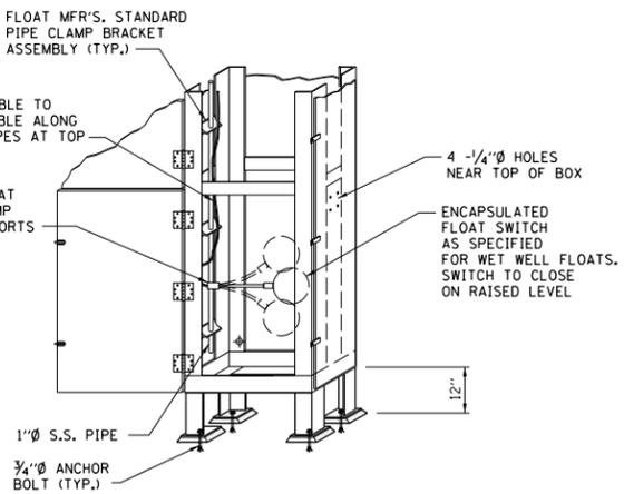
**ENLARGED FLOAT DETAIL IN STILLING WELL ENCLOSURES**
