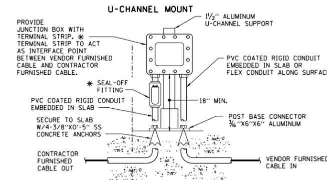
\* PROVIDE NEMA 7 EXPLOSION-PROOF JUNCTION BOXES AND SEALOFF FITTINGS WHERE CLASSIFIED OR CORROSIVE LOCATIONS ARE IDENTIFIED ON DRAWINGS.
