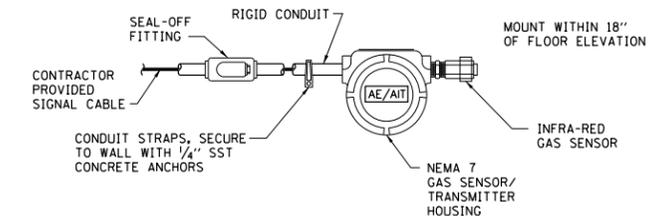
**COMBUSTIBLE GAS SENSOR/ TRANSMITTER-INFRA-RED N004**
