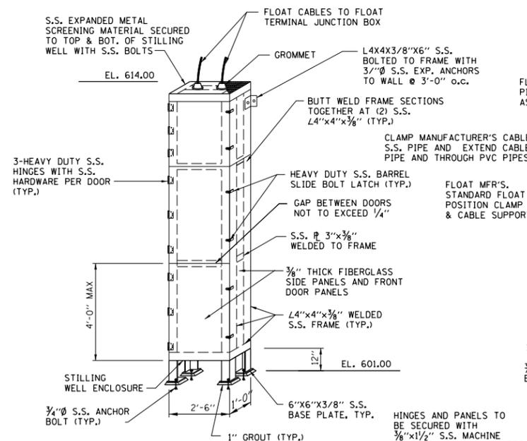
**FLOAT STILLING WELL DETAIL FOR PUMP FLOAT CONTROL**
