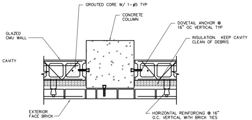
**MASONRY WALL ANCHOR DETAIL-S34**
