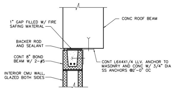
**INTERIOR MASONRY WALL ANCHOR DETAIL-S37**
