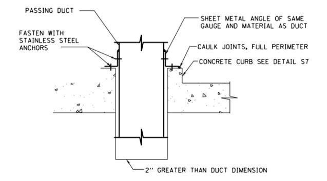
**TYPICAL DUCT FLOOR PENETRATION DETAIL**
