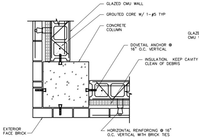
**MASONRY WALL ANCHOR DETAIL-S33**
