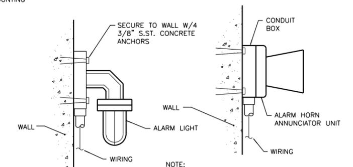
NOTE: PROVIDE SEAL-OFF CONNECTORS AS REQUIRED TO COMPLY WITH NEC REQUIREMENTS.
