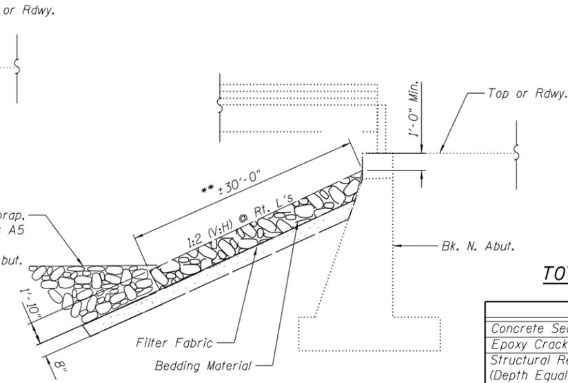
**PROPOSED SECTION THRU RIPRAP SOUTH ABUTMENT**
