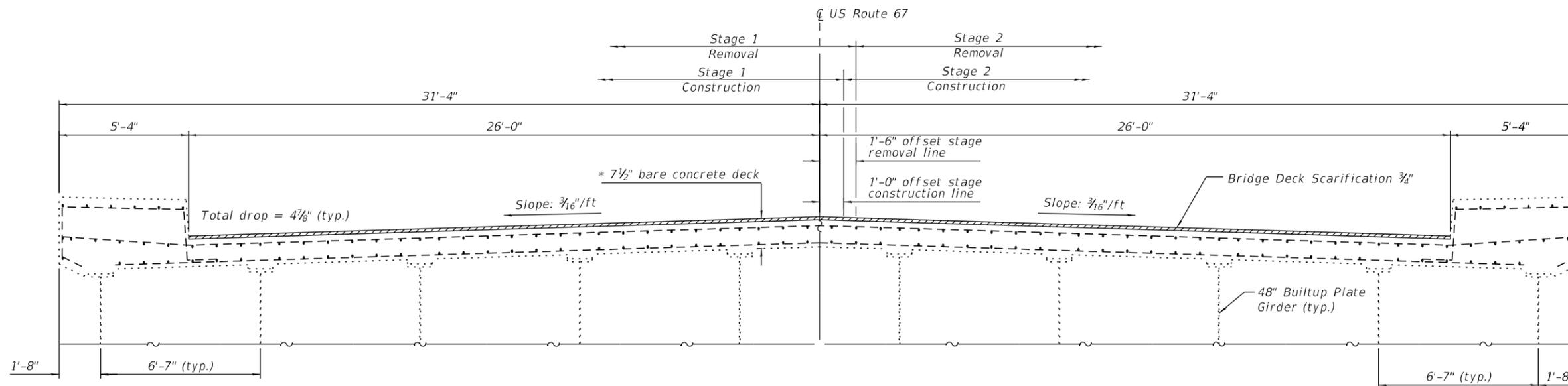
**CROSS SECTION SHOWING REMOVAL**
