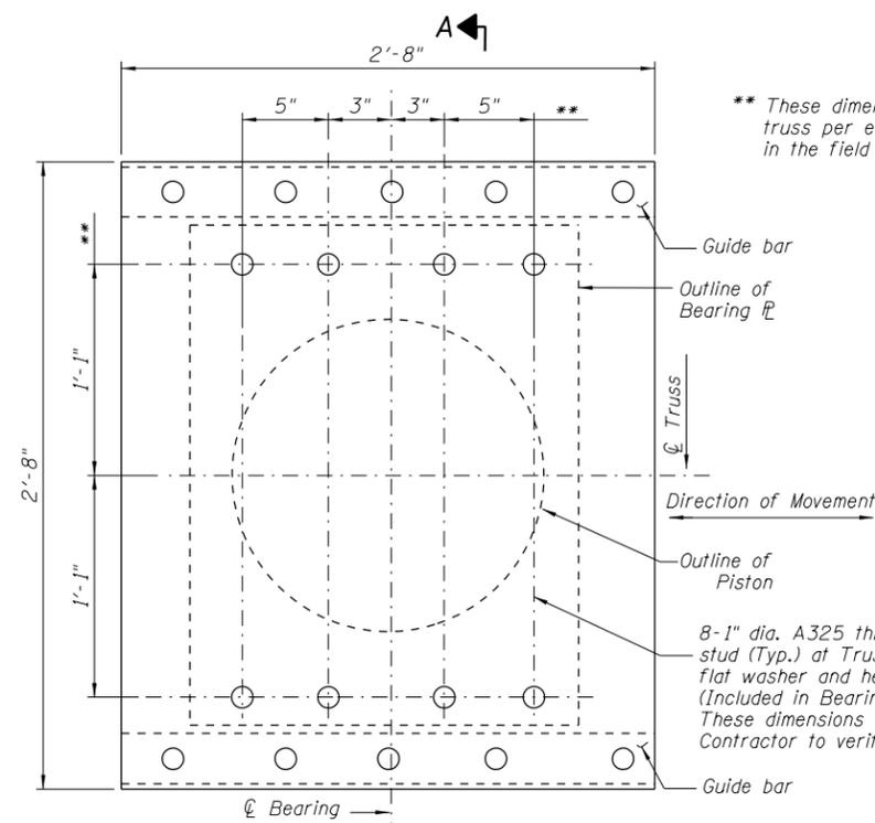
**TOP BEARING PLATE AND PISTON PLAN**
