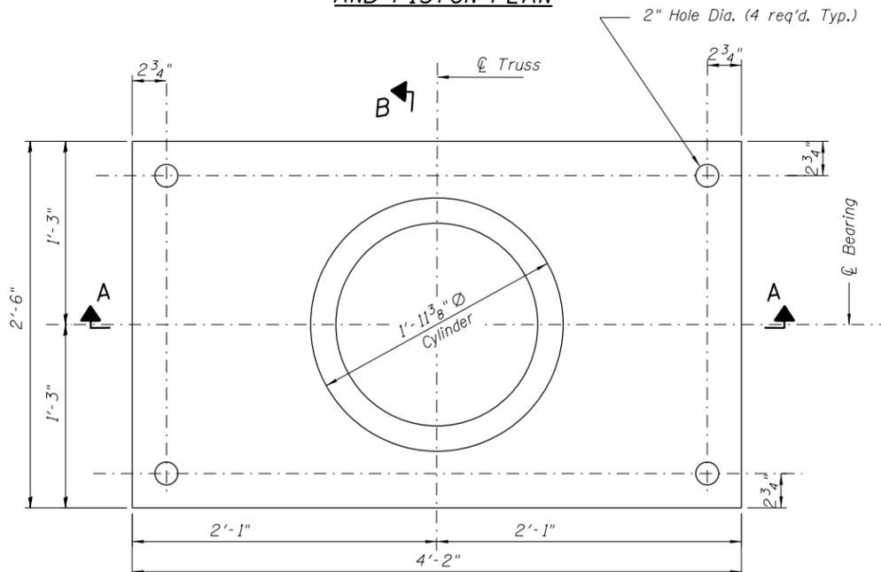
**BOTTOM BEARING PLATE AND BASE CYLINDER PLAN**
