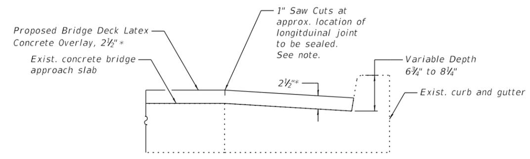
CURB AND GUTTER OVERLAY DETAIL
