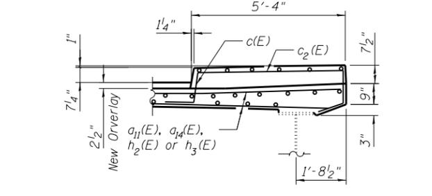
**PIER 1 TO SOUTH ABUTMENT TYPICAL SECTION AT SIDEWALK**
