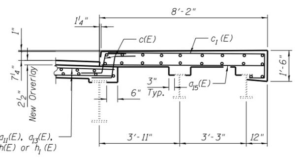
**NORTH ABUTMENT AND PIER 1 SECTION AT SIDEWALK**
