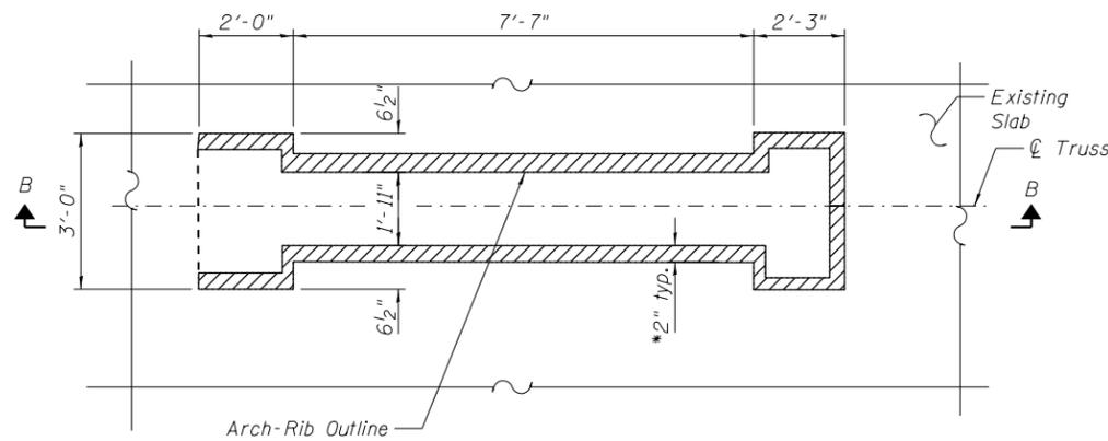
**TYPICAL PLAN VIEW OF ARCH-RIB**
