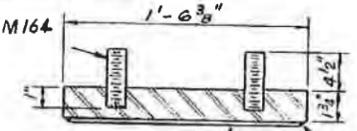
1/16" Stainless steel sliding plate, A240, Type 304, 2B finish.
