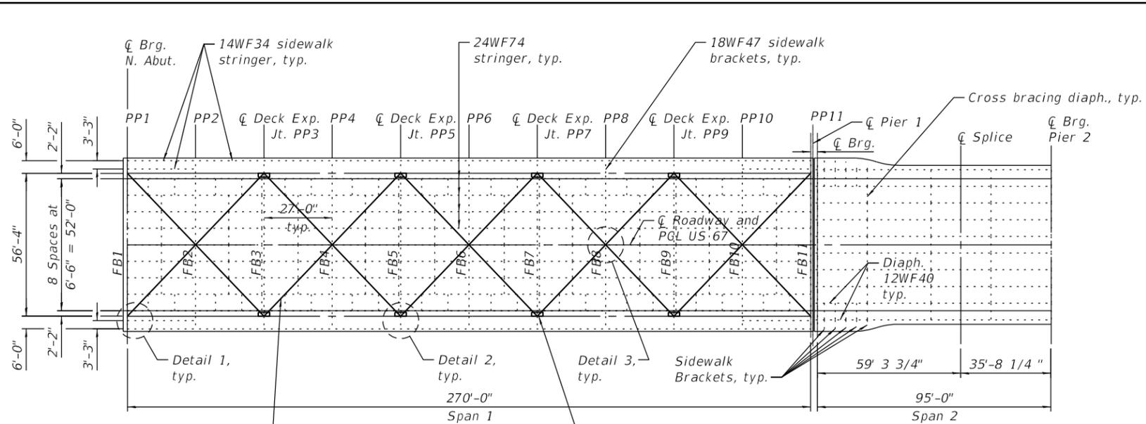
Bottom lateral diagonal bracing, 2 L's 5"x3 1/2"x3/8". Remove and replace at all deck expansion joint locations, twenty (20) locations total. Paid under Structural Steel Removal and Furnishing and Erecting Structural Steel, typ.
