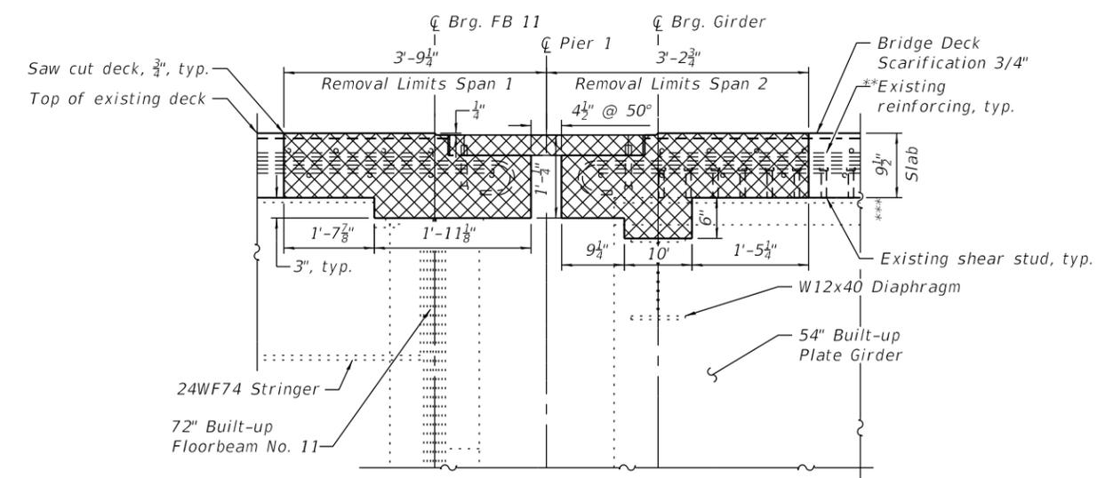
Any reinforcement bars that are damaged during concrete removal operations shall be repaired or replaced using an approved bar splicer or anchorage system. Cost incidental to "Concrete Removal".
