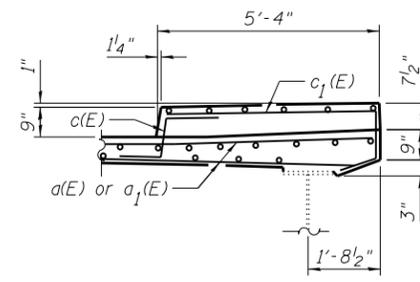
**ABUTMENT SECTION AT SIDEWALK**
