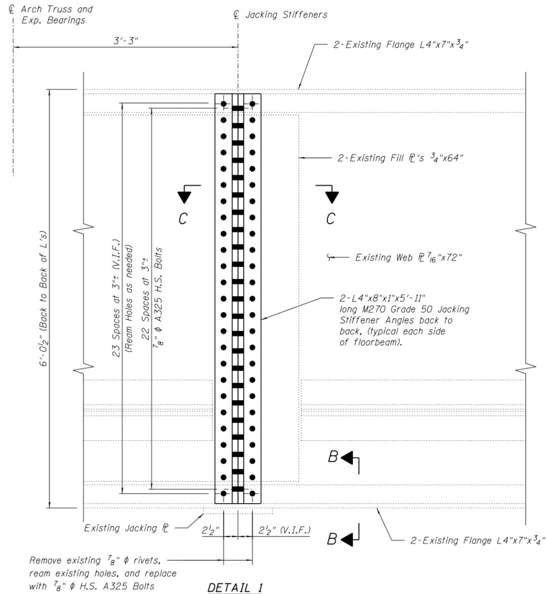
Remove existing 7/8" φ rivets, ream existing holes, and replace with 7/8" φ H.S. A325 Bolts
