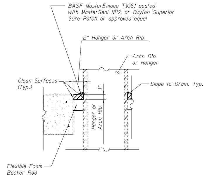
**TYPICAL SEAL SECTION DETAIL**
