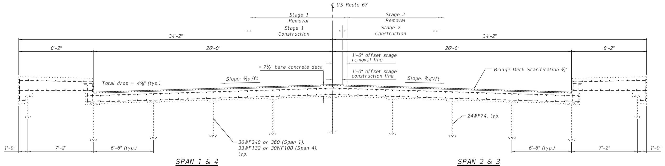
**CROSS SECTION SHOWING REMOVAL**
