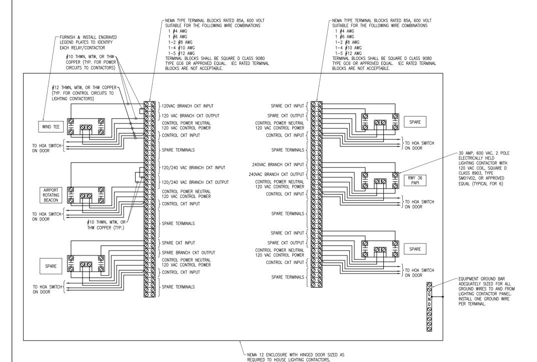
TERMINAL BLOCKS, WIRING & INTERFACE TO EXISTING
