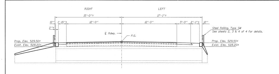
ELEVATION Note: Roadway dimensions shown are perpendicular to roadway.
