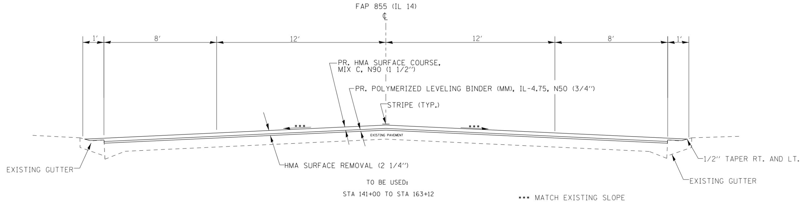
NOTE: HMA REMOVAL IN GUTTER AREAS SHALL BE INCLUDED IN HMA SURFACE REMOVAL, 2 1/4"
