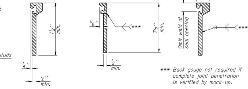
\*\*\* Back gouge not required if complete joint penetration is verified by mock-up.
