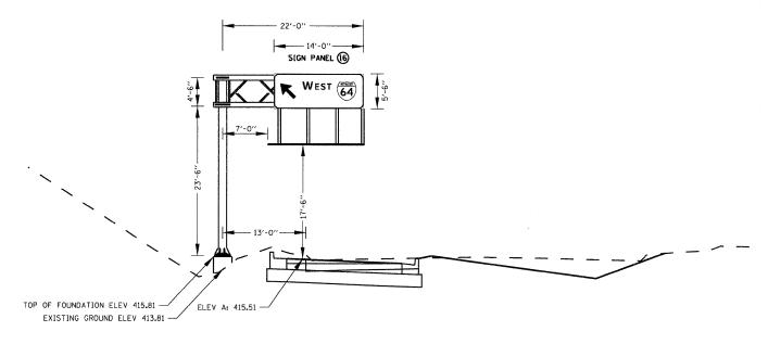
NOTE: CONTRACTOR SHALL LOCATE AND PROTECT EXISTING 36" STORM SEWER WHILE DRILLING SIGN FOUNDATION. COST TO BE INCLUDED IN COST OF CANTILEVER SIGN.
