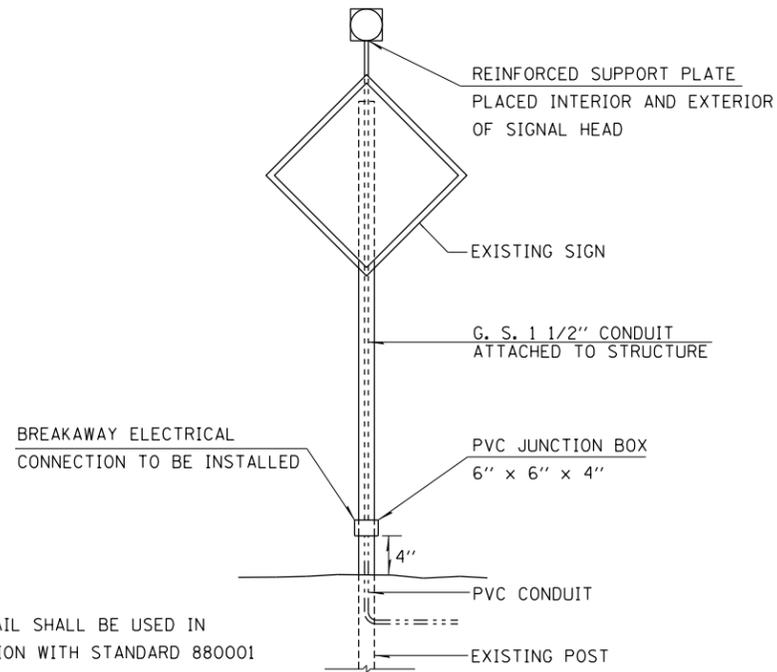
POST MOUNTED FLASHING BEACON
