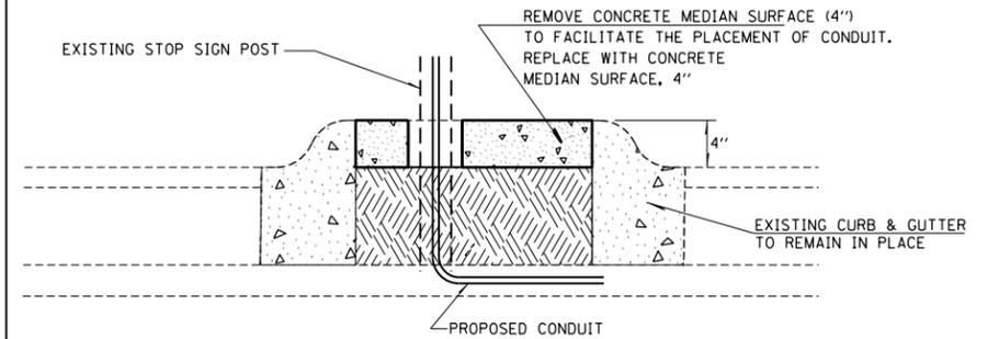
CONCRETE MEDIAN SURFACE, 4 INCH DETAIL
