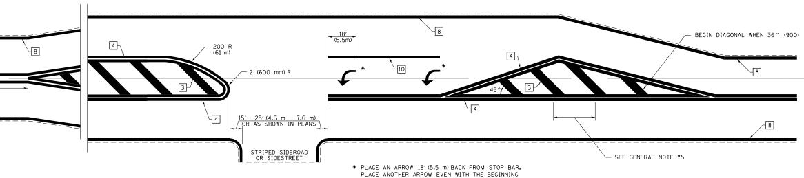
\* PLACE AN ARROW 18'(5.5 m) BACK FROM STOP BAR. PLACE ANOTHER ARROW EVEN WITH THE BEGINNING OF THE SOLID WHITE LINE. SPACE ADDITIONAL ARROWS EVENLY UP TO 80'(24.4 m) MAXIMUM SPACING. USE MINIMUM OF 2 ARROWS.
